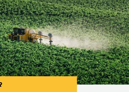
Four fans and Gearmore Venturi product delivery increases canopy movement and agitation for targeted spray coverage
