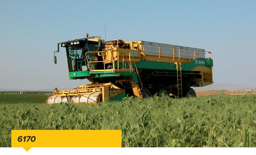
Oxbo is proud to introduce the next generation in pea, lima bean, and garbanzo bean harvesters. A new propulsion system eliminates the front four wheel motors and offers instead a mechanical 6 wheel drive option. With the availability of wheeled or track options, the Oxbo 6170 can fit the needs of all growers.
