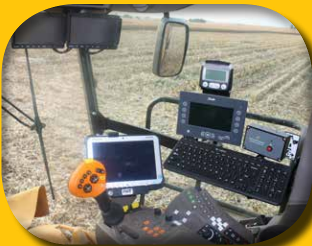
Technology functions: HarvestMaster MIRUS software is integrated directly into the Oxbo machine control system
