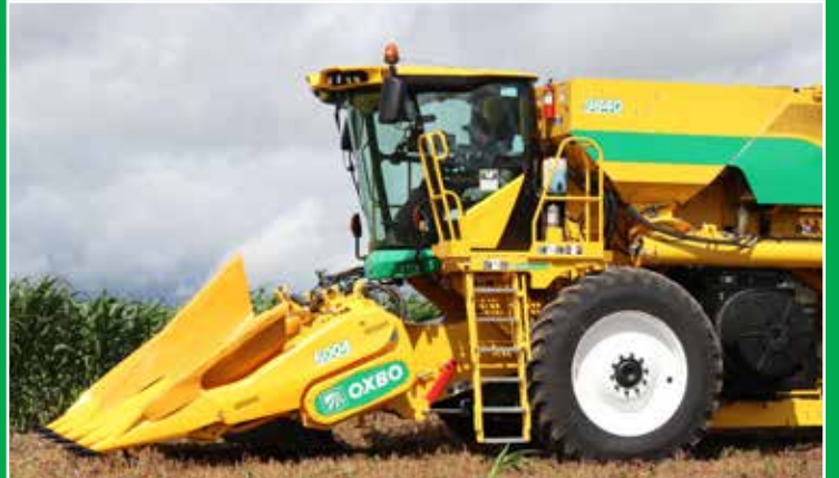
Easy access cab: Ladder retracts to keep width at a minimum
