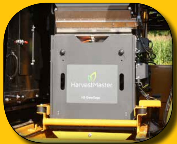
Oxbo Exclusive: HarvestMaster H2 GrainGage™ with tri-hopper quickly cycles through plots and reports data to MIRUS software for the most accurate results
