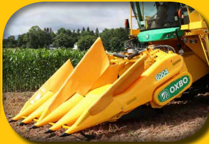
6004 chopping head: Chops residue into smaller pieces for increased decomposition
