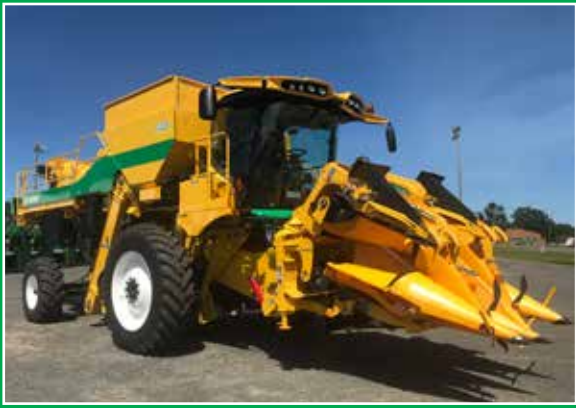
Dual-folding head: Four row head folds up for standard trailer width. No over-width permits required!
