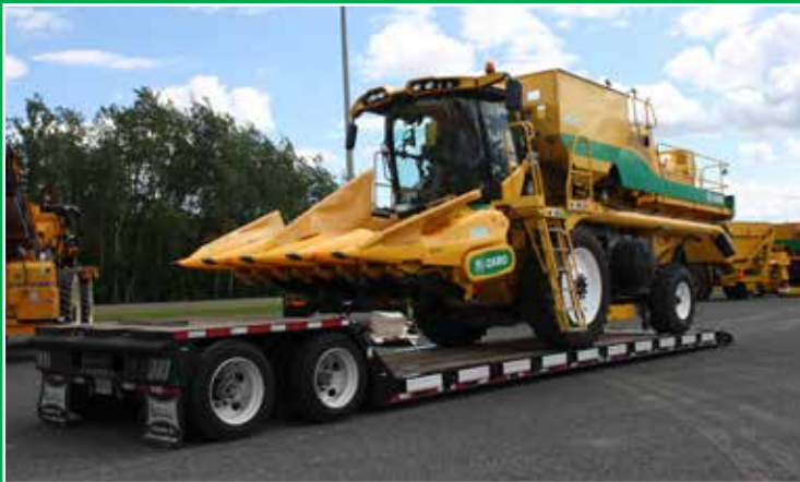
Drive on for transport: Axles slide in to narrow up combine to fit on standard trailer
