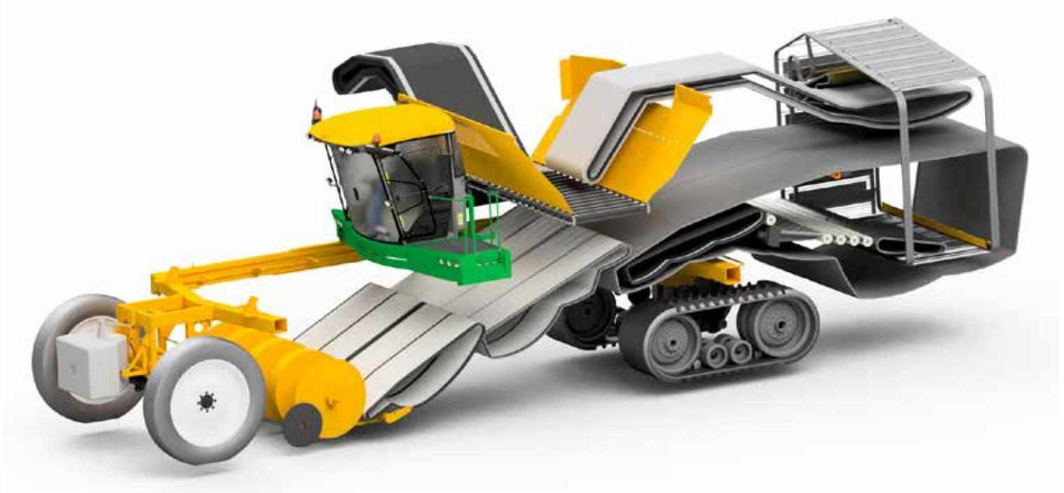
**TYPE 75.794** 3 sieving webs, axial roller system, PSHS system (4 rollers) and a de-viner belt
