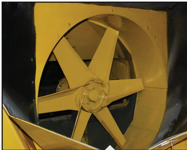
Powerful Suction Fan: Key component of IntelliClean, two-part cleaning process
