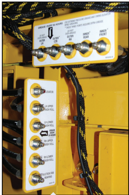
Serviceability: Centralized grease banks and easy access locations
