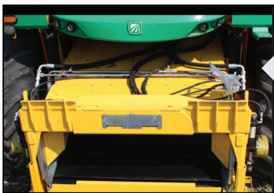
SoftTouch: Gentle crop handling through an entirely belted system
