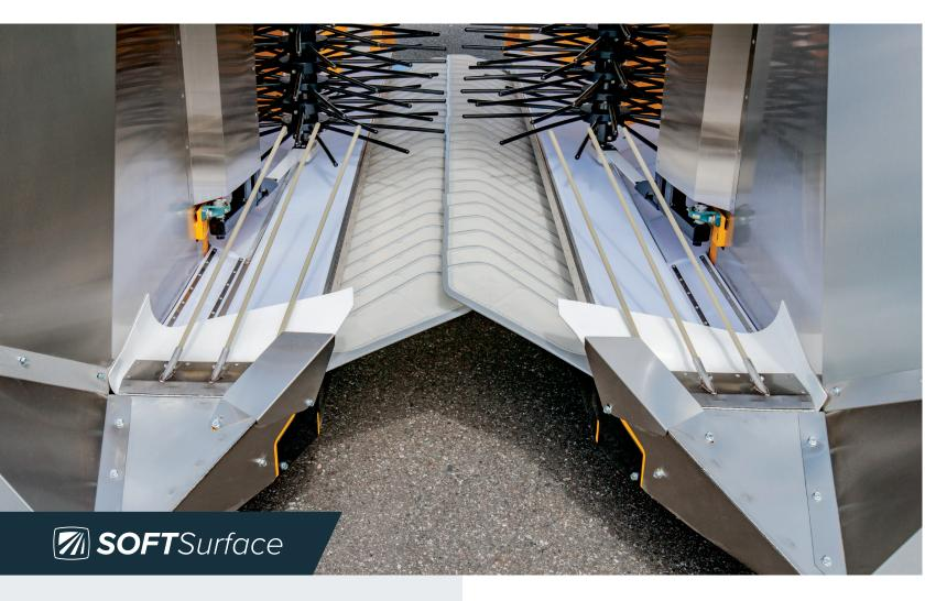
Compatible with the Oxbo 7440, 8040, 8140 and 7450 the Oxbo SoftSurface kit has proven to reduce internal bruise damage in mechanically harvested blueberries.
