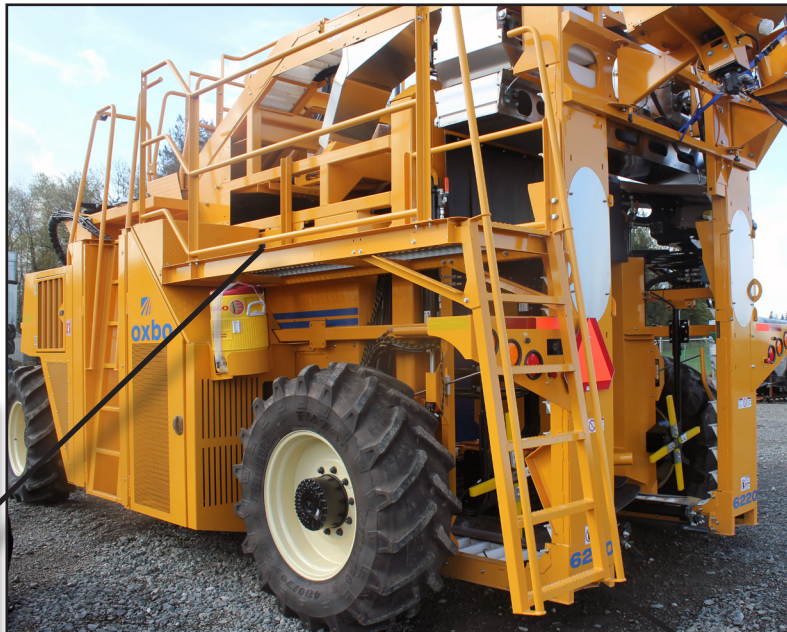
Bottom step on rear ladder flexes to be forgiving in the field.
