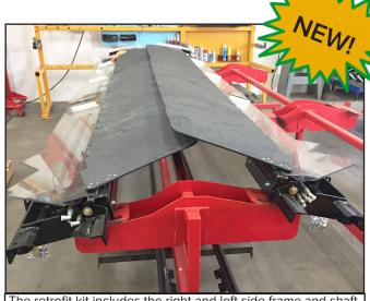
The retrofit kit includes the right and left side frame and shaft. (The kit does not include new motors)
