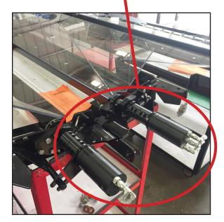
In the new design the shaker pan motor is set back into the frame with additional protection mounts.
