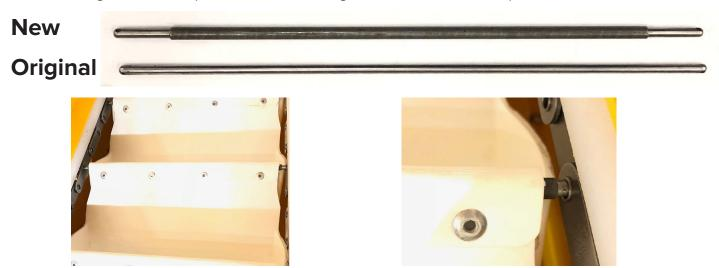
**Note:** the shoulder on the new pin is larger than the diameter of the hole in the chain and can not be inserted from the end. Therefore, the original pin is still valuable for quick, in-field repair during harvest.
