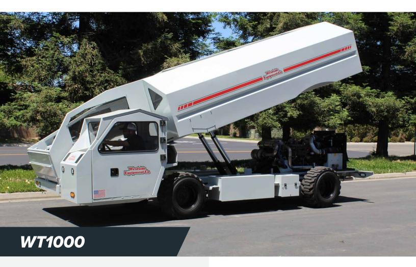
The bankout shuttle drives productivity with a top speed of 22 MPH. The air bag suspension delivers performance and comfort over the rough orchard terrain.
