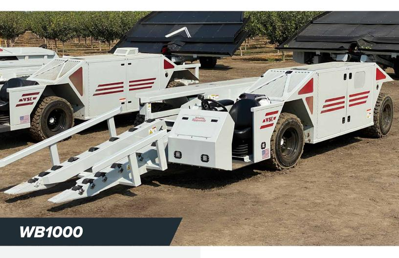
The bin carrier was designed for easy bin pickup with 16 roller forks including 14 chain-driven rubber rollers and two additional front idler rollers. Featuring joystick control, the bin carrier is easy to operate; buttons and switches are in easy reach.
