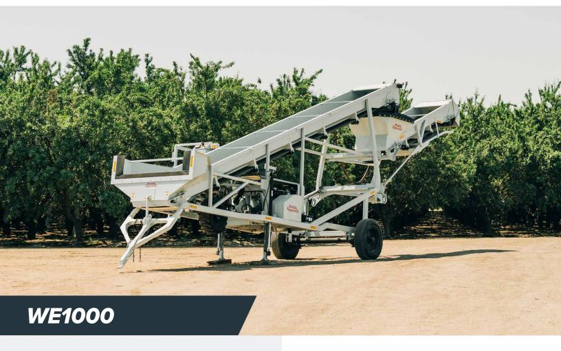
The elevator was designed for easy operation. Featuring joystick controlled powered front wheel steering, the elevator is easy to position and maneuver without additional assistance. The operator is ideally positioned to monitor all functions.
