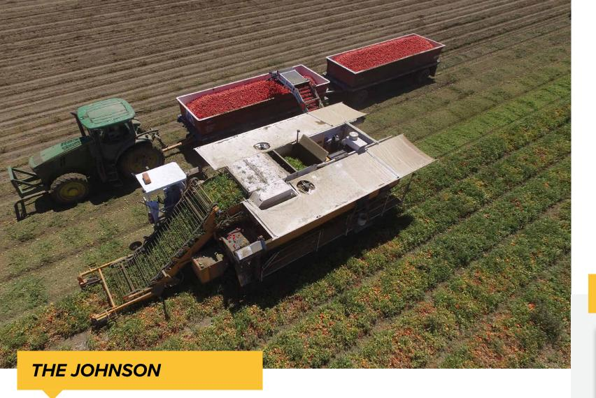
The Johnson Harvester is a heavier machine and a high performer in large open fields. Equipped with load sense hydraulics and independent flow controls for all functions, the Johnson is constructed with a heavy-wall tubular steel main frame that can withstand even the most adverse field conditions.
