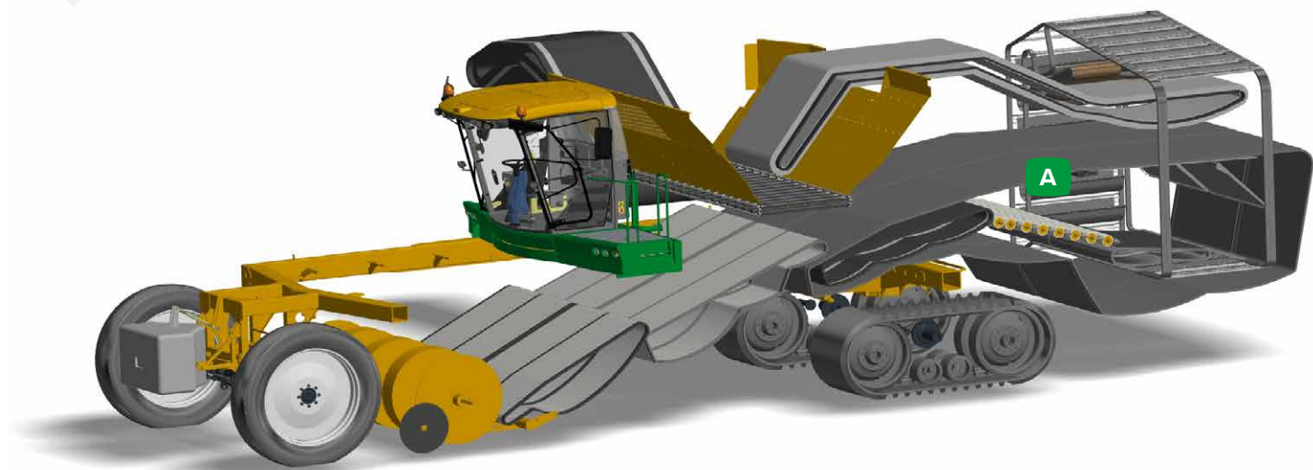
TYPE 76.790 3 sieving webs, PSHS system (8 rollers) and a de-viner belt
